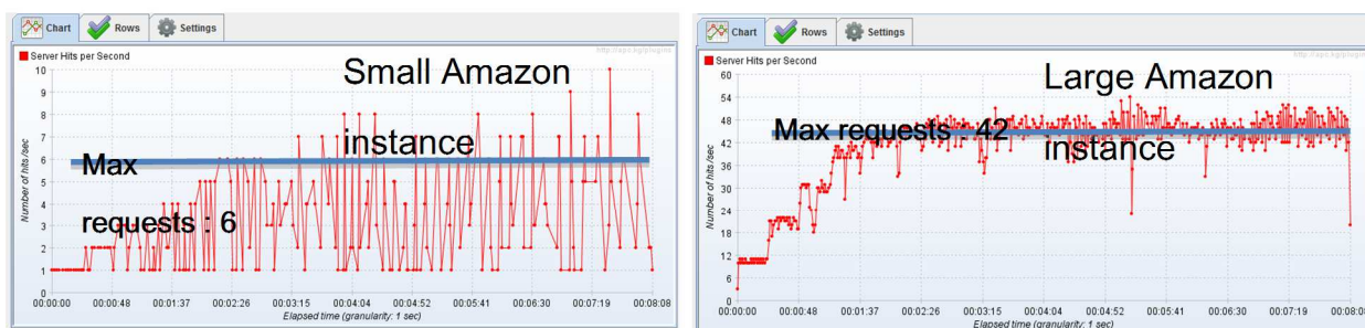
Figure 11: Comparison of two instances for a charge test of a GetMap operation
